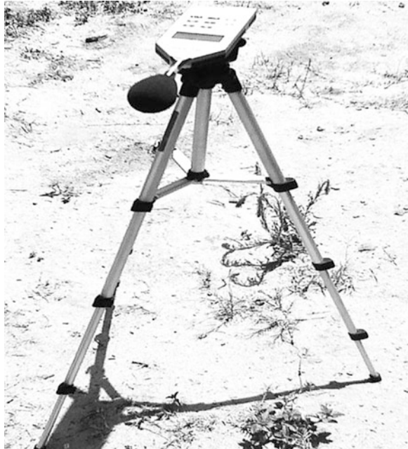
Fig. 1 Sound level meter on a tripod with windscreen
