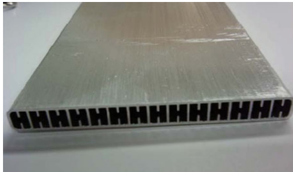
Fig. 7 Aluminum section of cold plate
