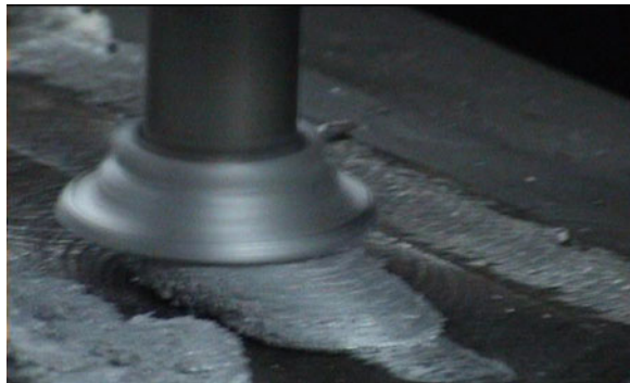
Fig. 3 Coating of aluminium over mild steel
