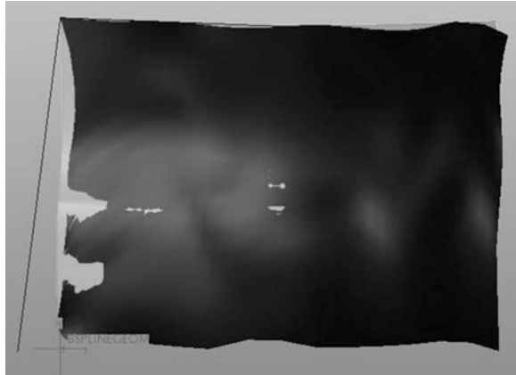
Fig. 12 Overlapping of B-spline machined and desired surface
