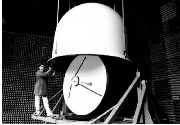
Fig. 1 Installation of radome over the antenna
