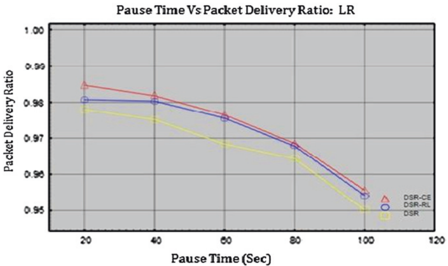
Fig. 2.4 Packet delivery ratio for network of 50 nodes for low resolution
