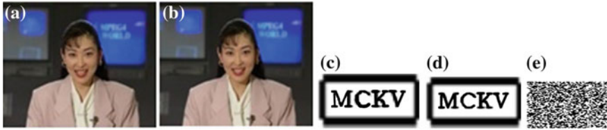
Fig. 11.1 a Original frame of Akiyo. b Watermarked frame of Akiyo. c Original watermark image ( 50 \times 25 ). d Extracted watermark ( 50 \times 25 ) from all watermarked video with NCC = 1 . e Extracted watermark using fake key. ( P, M, \epsilon ) above each image represents the PSNR (in dB), MSSIM and security values of the watermarked video frame. ( P : 43.99, M : 0.98, \epsilon = 0.0011 )
