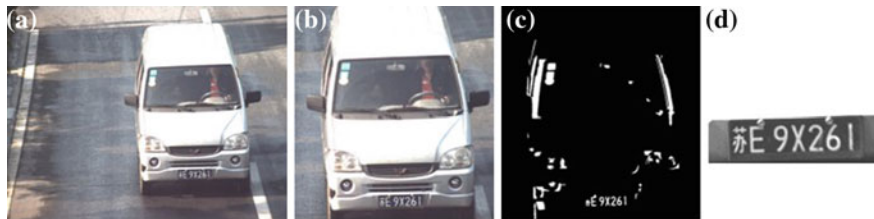
Fig. 3 a A raw image. b Detected vehicle. c Processed with top-hat transformation. d Localized license plate
