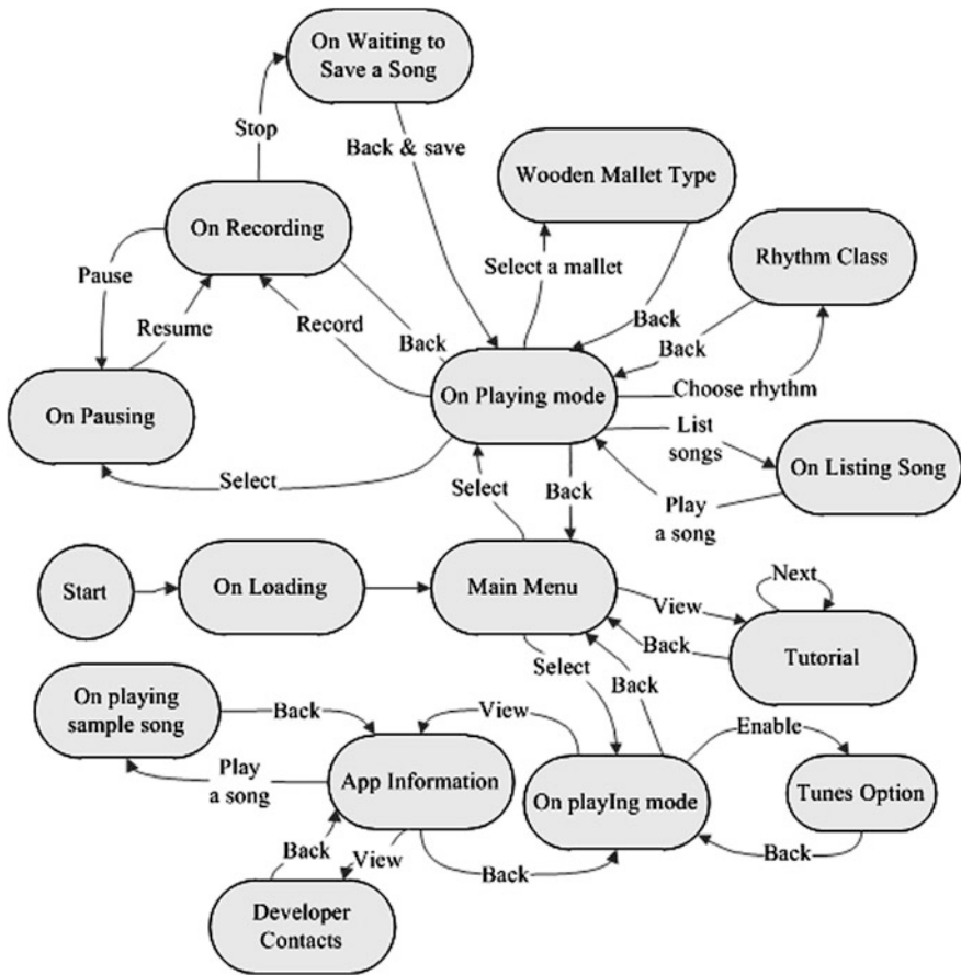
Fig. 8 The overview of improved-state diagram of the application
