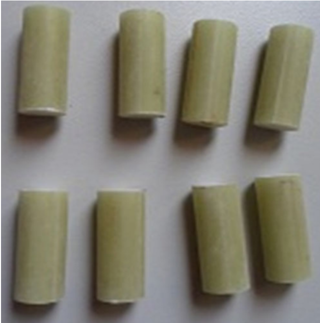
Fig. 1 Pin of pultruded GFEC (75 % glass fibre)
