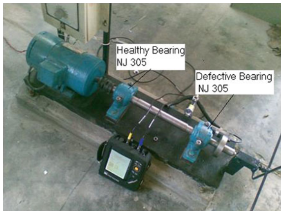
Fig. 5 View of experiment setup with Vibration Analyser, Experiment.rig
