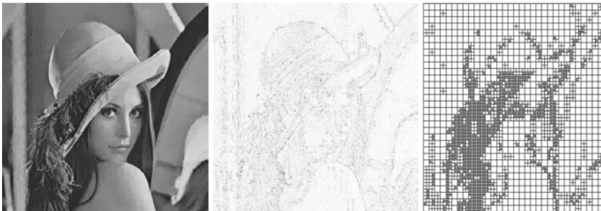
Fig. 4 Encoding results using PIFS partitioning scheme on GPU cluster (PSNR: 19.54, Compression ratio: 341.89 %)
