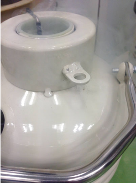
Fig. 9.5 Check for vapors emanating from the neck of the shipper on arrival
