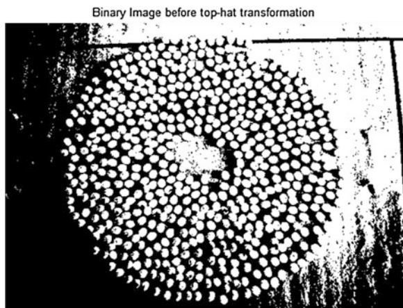
Fig. 4 Thresholding before applying top-hat filtering
