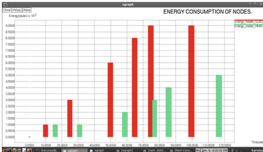
Fig. 5 It shows the energy consumption achieved using HMAC. This measures the energy expended per delivery data packet. It is expressed as
