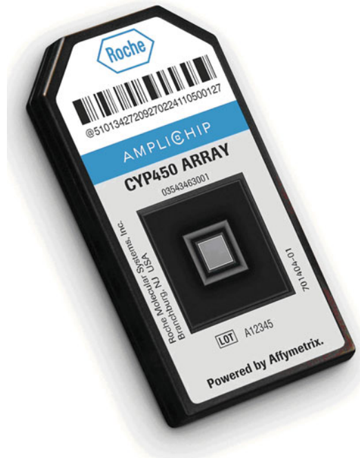
Fig. 22.3 The P450 assay chip for CYP2C19 genotyping (Reproduced with permission from Roche)
