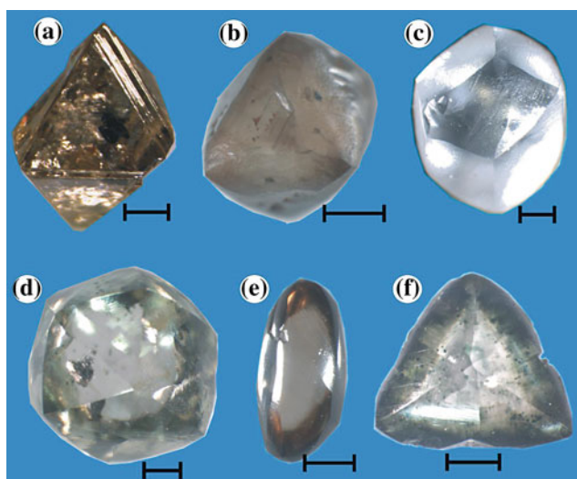
Fig. 5 Representative crystal forms of southern Indian diamonds. a Octahedron; b resorbed octahedron; c equant dodecahedron with rhombic faces; d equant dodecahedron with triangular faces; e flattened dodecahedron; f deltoid dodecahedron. Stones ( a ) and ( e ) are from kimberlites; stones ( b ) and ( c ) from conglomerates; and stone ( d ) is from gravels. Bar scale is 1 mm long
