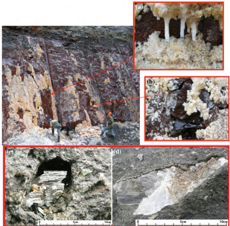
Fig. 4 a, b Deposition of modern halite in the Udachnaya open pit at the 450–480 m level in 2008; c, d geodes in a leached kimberlite partly (c) or completely (d) infilled with gypsum
