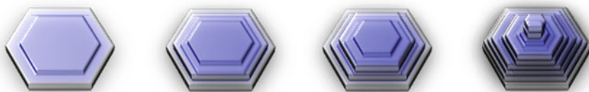
Fig. 1.16 Schematic representation of the formation of 1D nanowires on the 2D hexagonal stacking
