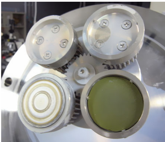
Fig. 7.3 Photograph of the multi-target changer
