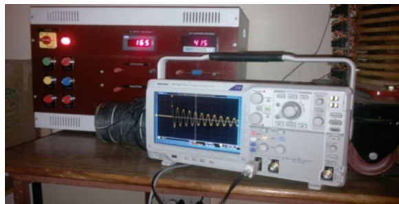
Fig. 5 Photograph of damped sinusoidal waveform generator with DSO
