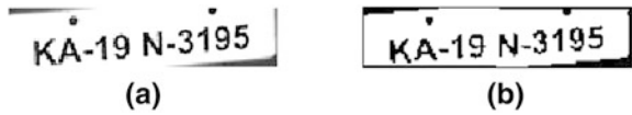
Fig. 5 Slant correction of extracted number plate a Slant detection b Slant correction
