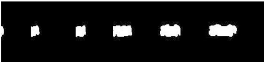
Fig. 6 Blobs from motion detection in a sequence of images showing the case of entry of a new object and revealing a series of occlusion state transitions of partial occlusion states before complete visibility
