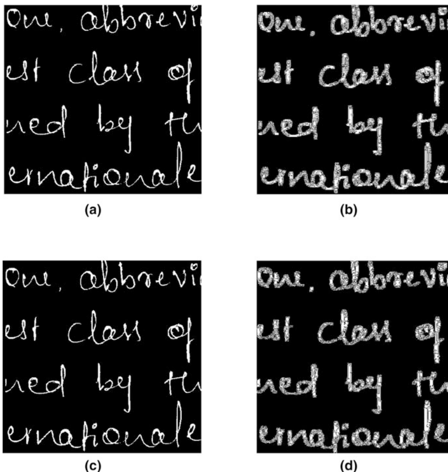
Fig. 3 Gabor filtered images for 0^\circ , 30^\circ orientations with frequencies 0.5. a Binary Image. b Gabor output for 0^\circ and frequency 0.5. c Binary Image. d Gabor output for 30^\circ and frequency 0.5
