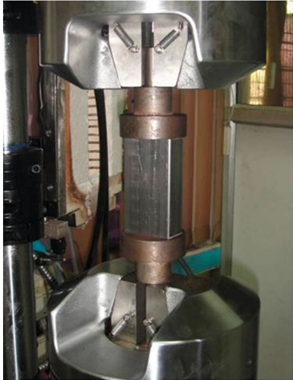
Fig. 5 Photograph of crush test of foam filled extruded section
