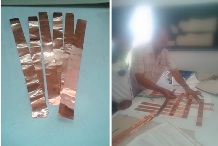
Fig. 2 Copper strips used for heat transfer and placed in the fabric
