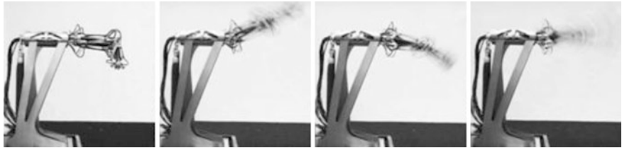
Fig. 18 Maximum acceleration 12 g, maximum velocity 11 m/s. Source scionic® I.D.E.A.L.
