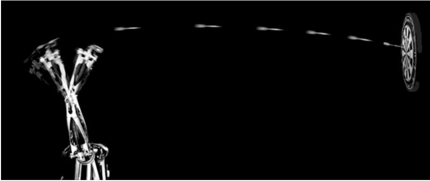
Fig. 19 Airarm throwing dart. Typical power consumption of 600 W, maximum 2,500 W. Source Univ.Prof. Dr.-Ing. (habil.) Christoph Ament
