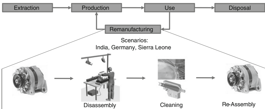
Fig. 2 Sustainability expert’s view on different remanufacturing scenarios of an alternator (assessment of processes and location regarding Global Warming, child labor etc.)
