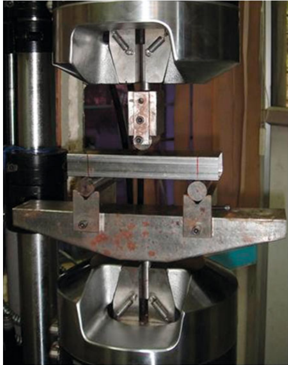
Fig. 6 Three point bend testing of foam filled extruded sections
