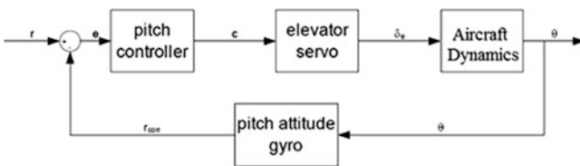
Fig. 30.2 A pitch attitude autopilot system
