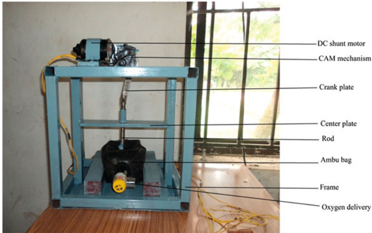
Fig. 35.2 Front view of the developed project
