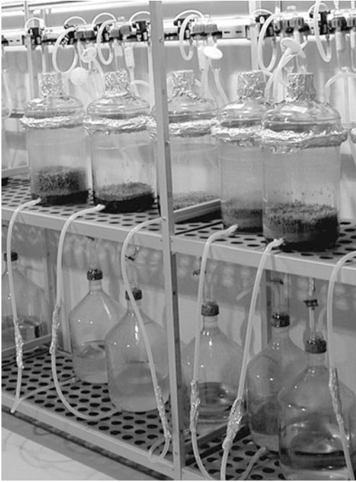
Fig. 7.7 Temporary immersion bioreactors used for mass multiplication of coffee embryos. The culture vessels on the top shelf are connected with the medium reservoirs on the lower shelf. (courtesy Jean-Paul Ducos Nestlé R & D Center–Tours, France)
