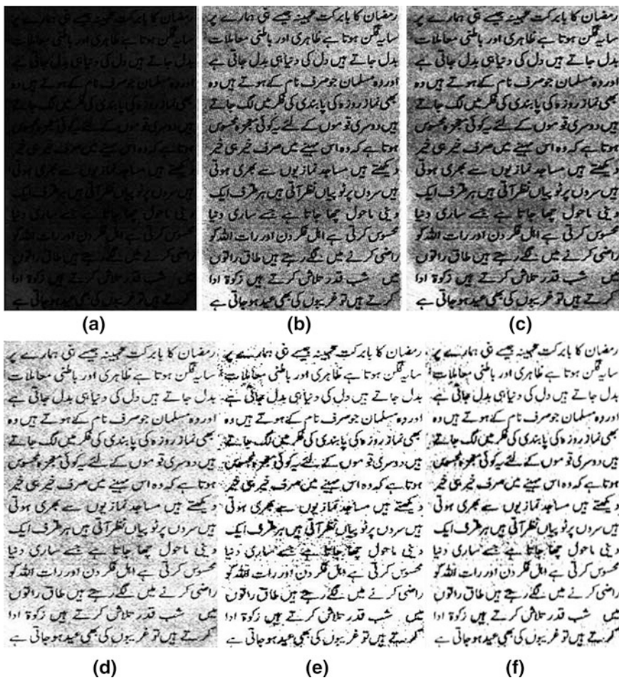
Fig. 3 a Original image. b Histogram equalized image. c 3 \times 3 median filter of image b. d 3 \times 3 max filter of image b. e Thresholded image of d. f Frequency domain Gaussian filter of image e
