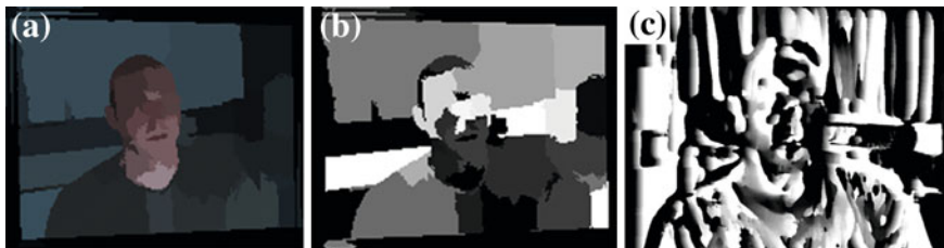
Fig. 3 a Homogeneous region obtained by color segmentation, b Disparity map of proposed method and c correlation based Sum of absolute difference
