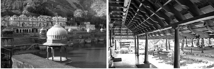
Fig. 3 Traditional tropical architecture of the last centuries was aware of the importance of solar shading in combination with natural lighting and ventilation. Depending on the climate zone, massive or wooden construction was preferred
