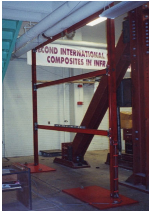
Fig. 2 Experimental verification of a scaled 2D frame
