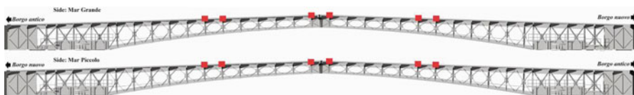
Fig. 10 Optimal sensors placement according to EFI method (12 sensors)
