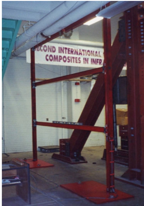
Fig. 2 Experimental verification of a scaled 2D frame
