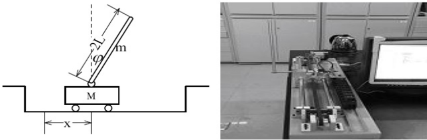
Fig. 1. (a) Inverted pendulum system sketch (b) Real time control effect picture of IP[2]
