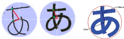
Fig. 6. The distance between COG and some of the pixel in target image (left) and that of the template image (right) for the Japanese character “あ” are shown
