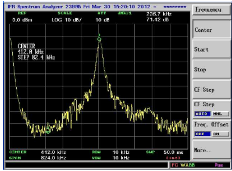
Fig. 8. Real time spectrum of BP filter output during flight
