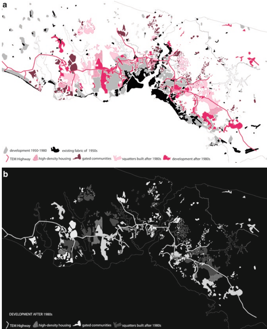
Fig. 10-7. (a) Fragmented hinterland of Istanbul (Mapping by Neyran Turan). (b) The development of Istanbul after the 1980s in relation to the TEM (highway). The map shows built fabric after 1980 and also depicts high-density housing (mostly developed along the TEM), squatter areas and gated communities. (Mapping by Neyran Turan)
