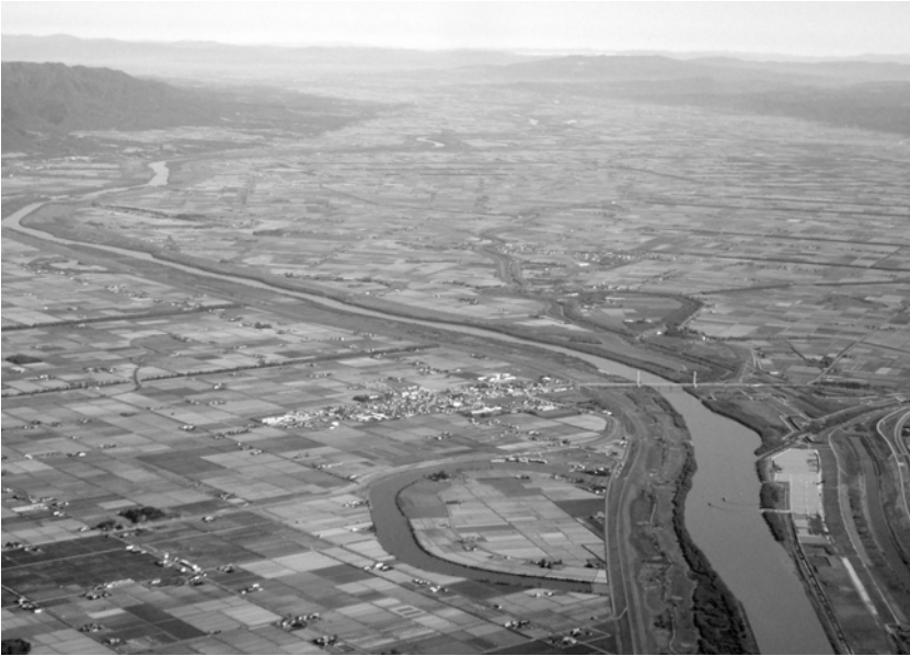
Fig. 6. Straighten channel at downstream of Ishikari river, Hokkaido. This river used to be 356km meandering channel has shortened to 268km after work
