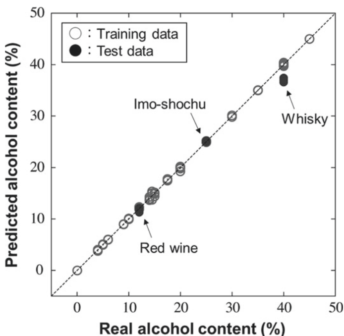
Fig. 6 Alcohol content prediction of liquors based on their smells: open and closed circles correspond to training and test data, respectively
