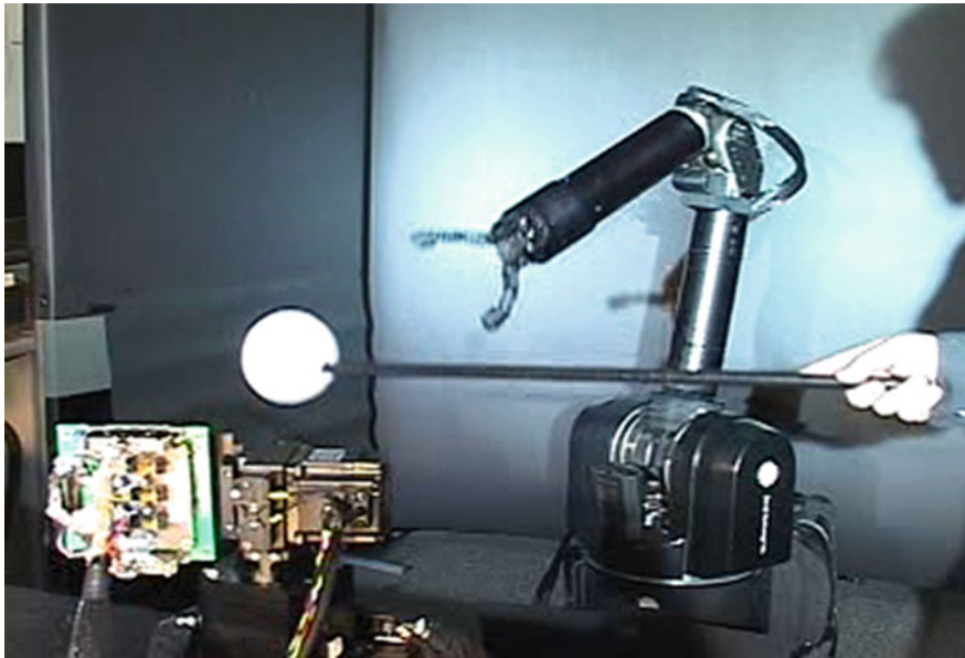
Fig. 9.3 Visual feedback control system (lower left in the photo is a tracking camera which captures a position of a white ball in front which is attached to the tip of a rod moved randomly by a person. And a black-colored hand-arm robot is controlled by a hard real-time control system aimed to grab the ball quickly)
