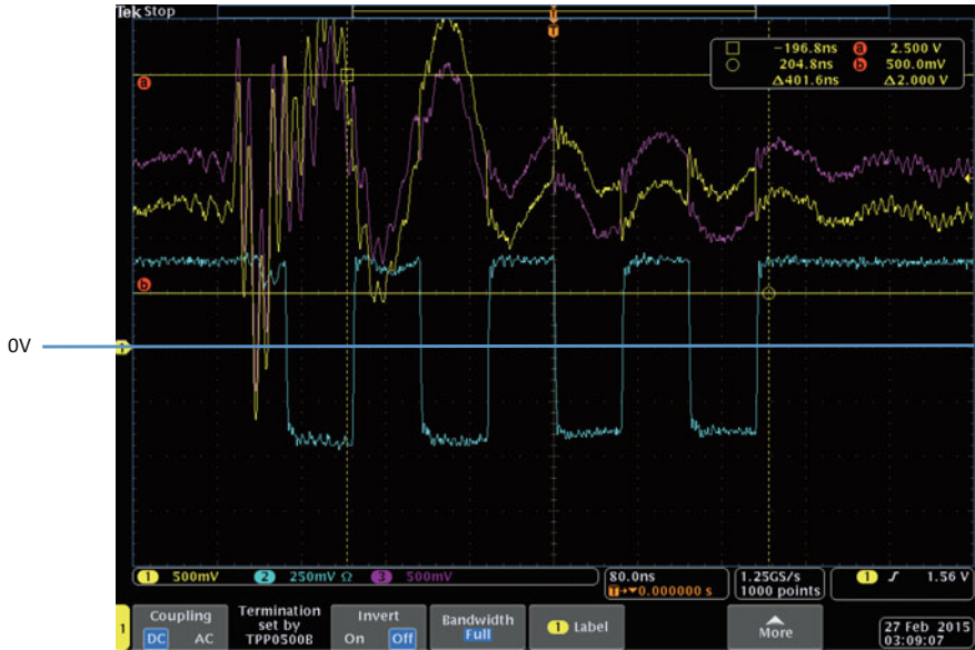
Fig. 4.32 Communication failure without ferrite core
