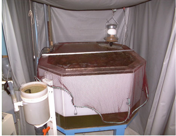
Fig. 4.2 Culture tank and sludge collector (front left)
