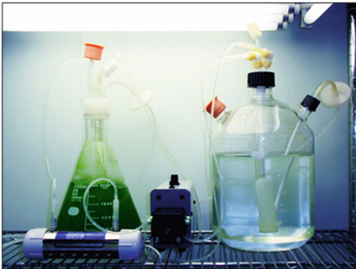
Fig. 13.5 A nutrient feedback rearing system for water fleas. The system was constructed using an algal cultivation flask (left side) (Cited from Endo and Takeuchi 2013)
