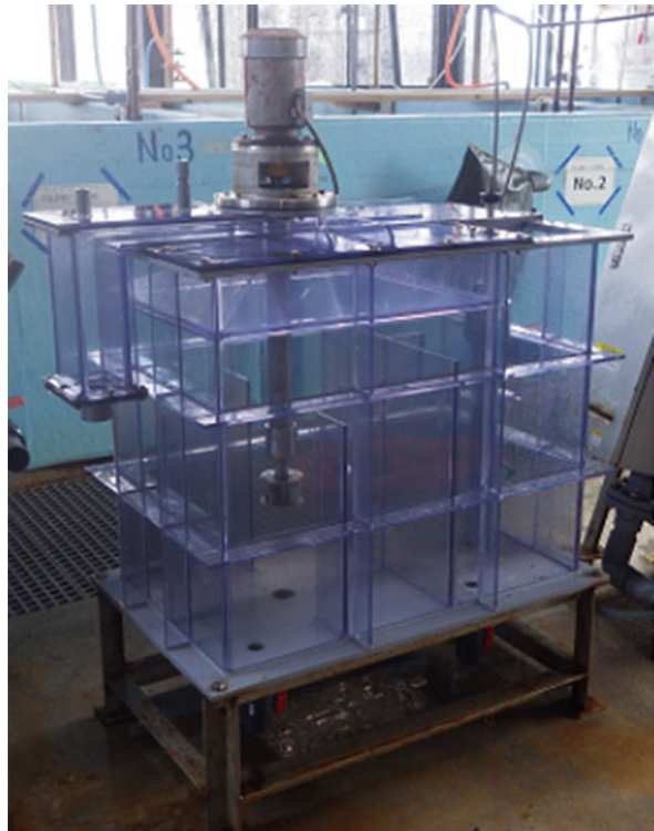
Fig. 2.6 Setting of KA-type foam separation unit in CRAS at Yashima Station in FRA
