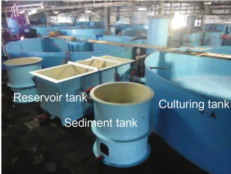
Fig. 2.3 Sediment tank in CRAS at Okinawa Prefectural Sea Farming Center
