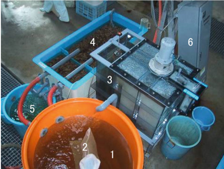
Fig. 9.4 Setting of prototype CRAS for seed production of Yashima station in FRA: 1, reservoir tank; 2, collection nets; 3, foam separation unit; 4, biofilter unit; 5, water level control tank; 6, UV sterilization unit
