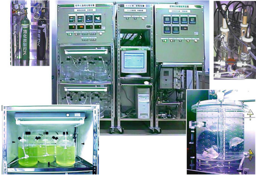
Fig. 13.6 Experimental unit for gas exchange between microalgae and fish
