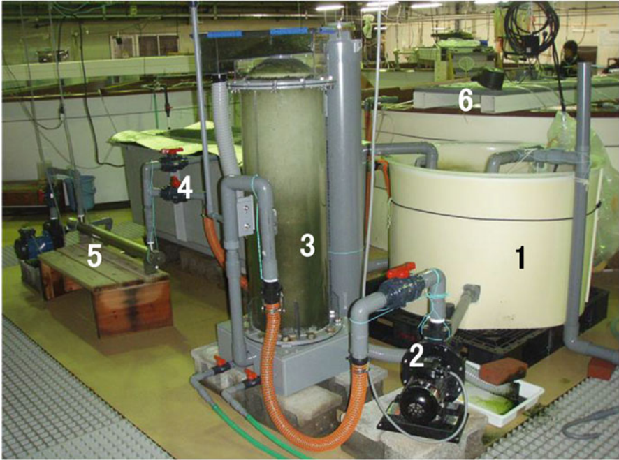
Fig. 9.15 Setting of practical type CRAS for seed production at Hiroshima Prefecture, Fisheries and Marine Technology Center (practical type system was developed by Yashima station in FRA): 1, reservoir tank; 2, recirculation pump; 3, foam separation unit; 4, biofilter unit; 5, UV sterilization unit; 6, rearing tank
