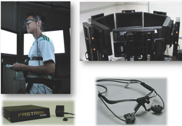
Fig. 5.2 The experiment was performed in a dark room using six 32-inch liquid crystal displays, arranged in the shape of a regular hexagon. Eye-in-head movements were recorded by an eye tracker, and head and body movements were recorded by an electromagnetic motion tracking system
