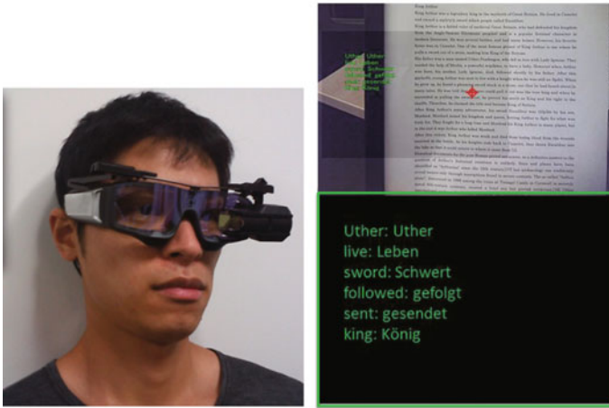
Fig. 7.20 Display of annotation by using a mobile eye-tracker and a head-mounted display
