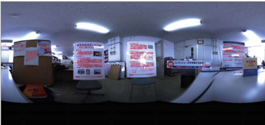
Fig. 7.8 Text detection by an omnidirectional camera
