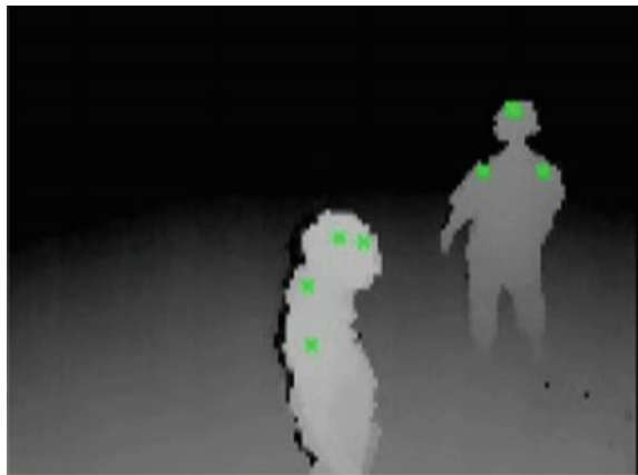
Fig. 4.5 Feature retrieval from depth images: green points represents shoulders and top of head
