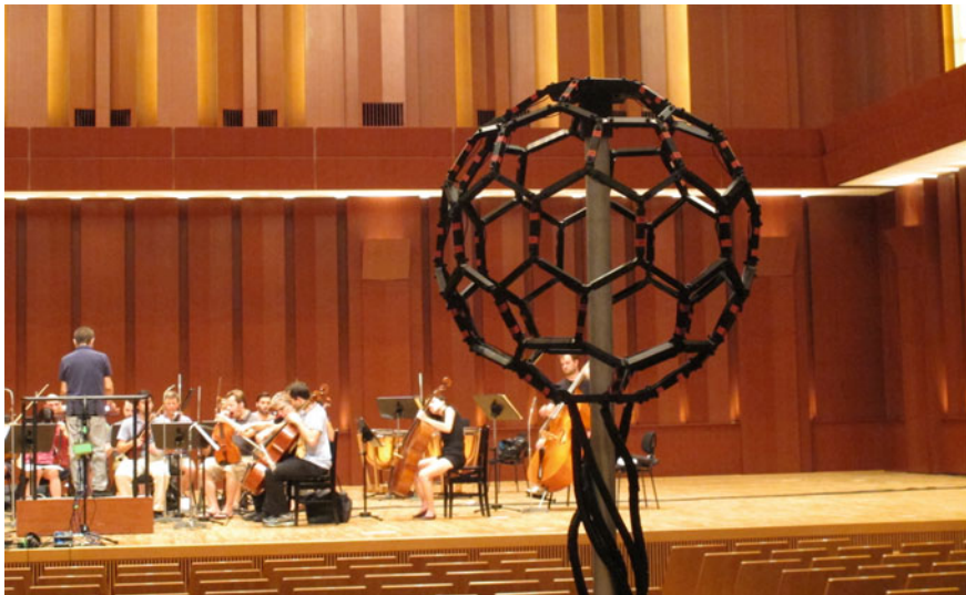
Fig. 2.2 3D sound field recording in a concert hall using a C80 fullerene microphone
