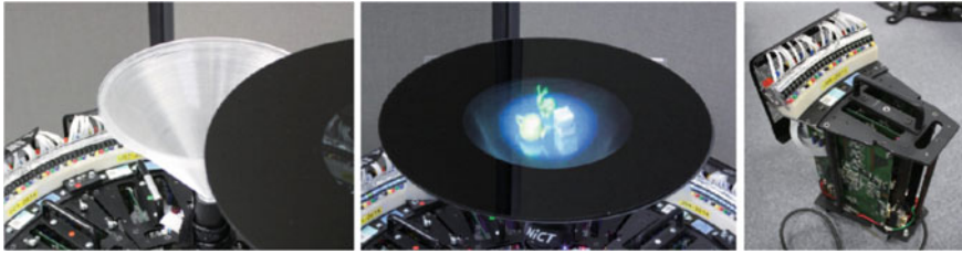
Fig. 6.22 Circularly arranged projectors and conical screen ( left ). The screen is covered by a semi-transparent black plate , and then a 3D image has appeared ( middle ). One projection module covers 30^\circ of viewing area. All together, 12 modules accomplish production of the 360^\circ -view 3D images ( right )
