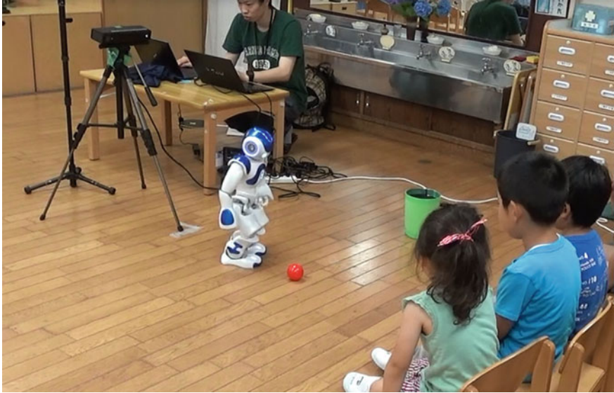
Fig. 8.11 Experimental environment: kinect sensor monitors positions of robot (NAO), ball, and children
