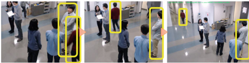
Fig. 5.23 Successfully suppressed false detection using gesture detection
