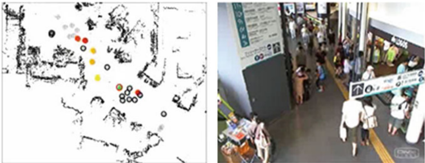
Fig. 4.14 Congestion where pedestrians pass through corridor's narrow part: left simulated scene, right actual scene
