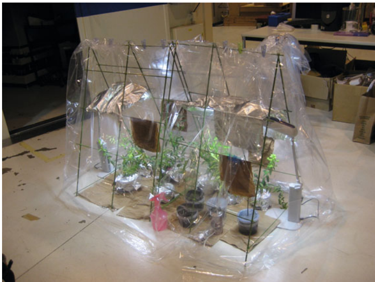
Fig. 6.10 Photograph of the “Green house,” temporarily placed along a beamline. \mu -XRF analysis of the willow plant requires maintenance of living plant materials in the synchrotron radiation facility, such that they are available for sample preparation. A wet cloth or spray will maintain moderate humidity. Plastic or aluminum lids on the pot cultures were designed to avoid the scattering of soil particles. The fluorescent lamps should be set carefully so that electricity does not leak
