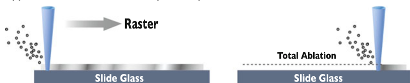
Fig. 4.1 Schematic diagram of sampling depth after the laser ablation. The resulting sampling depth can vary when the heterogeneous sample was ablated (a). With the conventional laser ablation, not only biological samples but also glass substrate was ablated (b). With the laser beam of reduced fluence (soft ablation protocol), only the sliced biological tissue samples could be preferentially ablated (c). This is very important to control the weight (volume) of sample ablated and also to minimize the contamination from glass substrate
