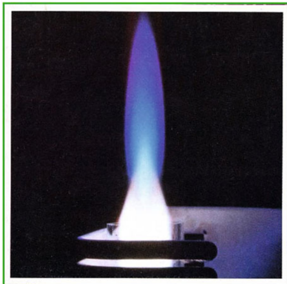
Fig. 1.1 A photo of an inductively coupled argon plasma used for excitation and ionization sources in ICP-AES and ICP-MS, respectively
