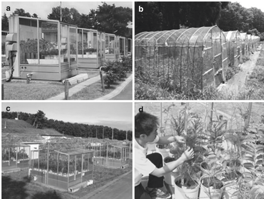
Fig. 5.1 (a) Naturally lit environmental control chambers, (b) greenhouse-type chambers, (c) open-top chambers, and (d) growth measurement of the seedlings in the open-top chamber
