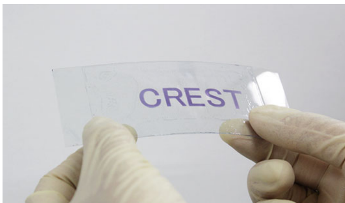
Fig. 12.5 A flexible solid-state electrochromic device using a polyFeL1 film
