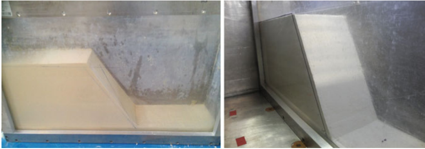
Fig. 3 The slope model with a 60° slope angle
