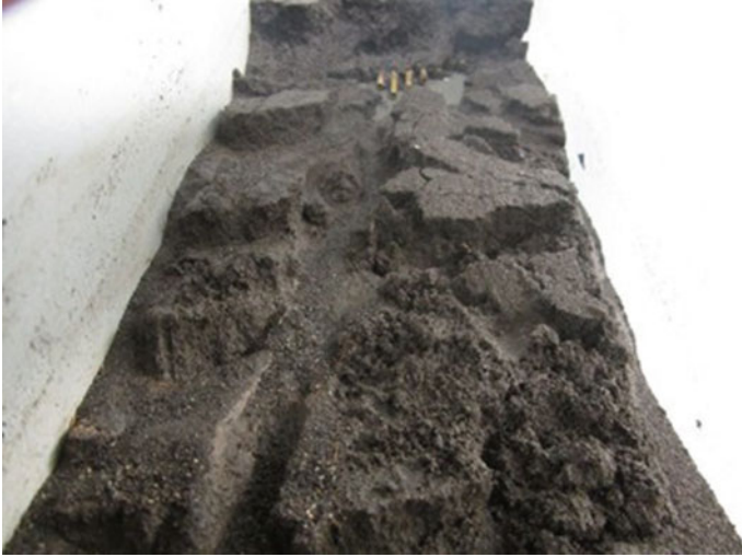
Fig. 15 Photo of damaged model slope after centrifuge test
