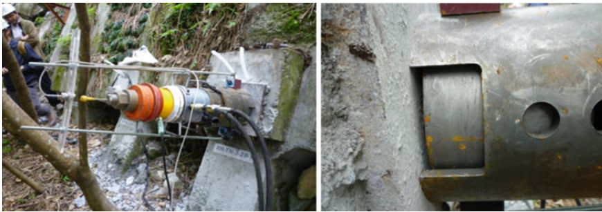
Fig. 9 Lift-off test for determining the residual anchor load
