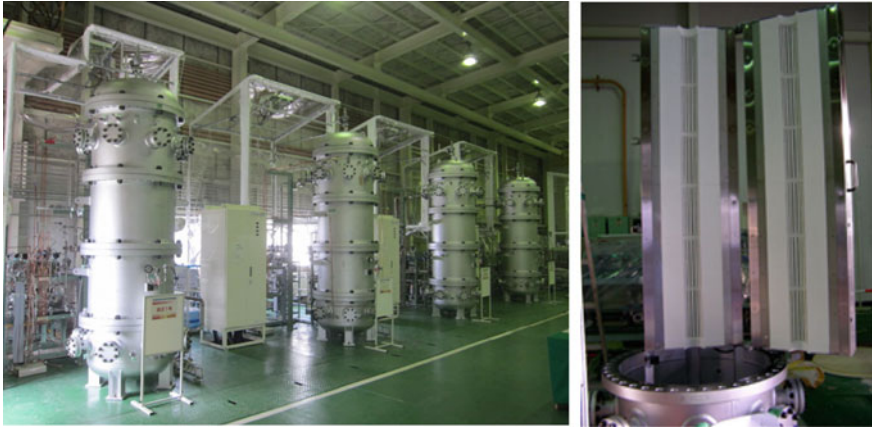
Fig. 37.7 Test apparatus of segmented-in-series tubular type cell stacks under high pressure
