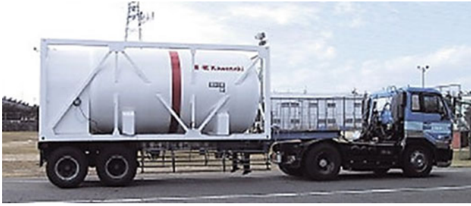
Fig. 4.13 LH 2 20 ft container (Kawasaki Heavy Industries)
