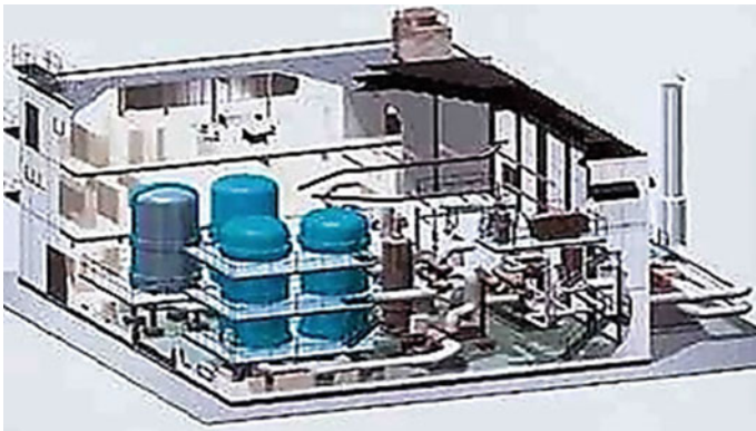
Fig. 5.20 Molten carbonate fuel cell (MCFC) 1 MW test plant. Source FCDIC
