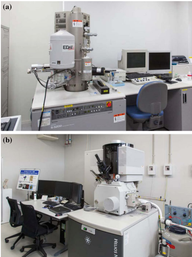
Fig. 21.13 Scanning electron microscope ( SEM ) equipped with a energy-dispersive x -ray ( EDX ) spectrometer and b focused ion beam ( FIB )
