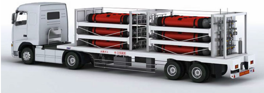
Fig. 19.4 Hydrogen trailer using 45 MPa high-pressure tanks [3]
