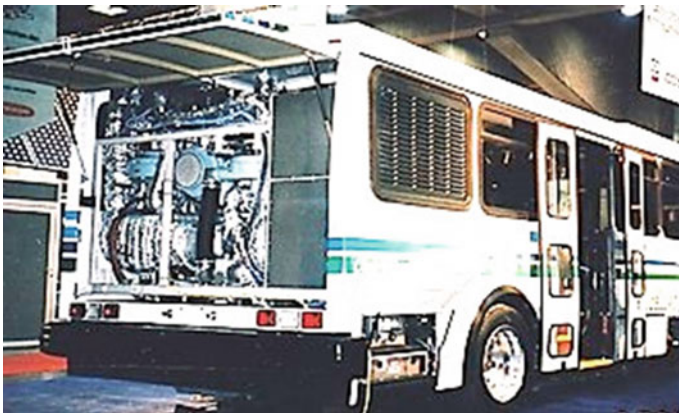
Fig. 4.41 Phosphoric acid fuel cell (PAFC)-mounted fuel cell bus
