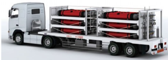
Fig. 4.29 45 MPa carbon fiber-reinforced plastic (CFRP) composite vessel trailer (Source Kawasaki Heavy Industries)
