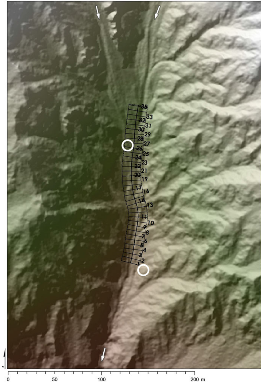
Fig. 8.5 Target area for terrestrial laser scanning. The background hillshade image is derived from an airborne-laser derived DEM with a resolution of 1 m provided by MLIT. Transverse cross section lines (20 m long) are set along the longitudinal section of the valley centre (170 m) at a spacing of 5 m. Two white circles indicate the approximate scan positions of the TLS. Arrows show the flow directions of major channels
