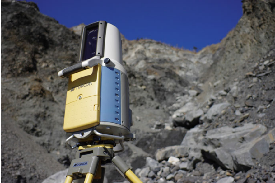
Fig. 8.4 Terrestrial laser scanner used in this study, GLS-1500 by Topcon Co.
