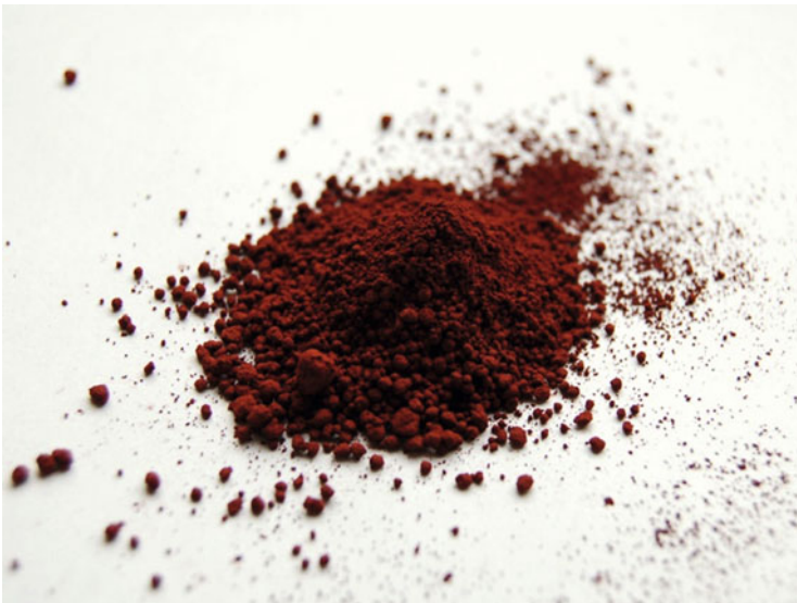
Fig. 1 Iron rust sample
