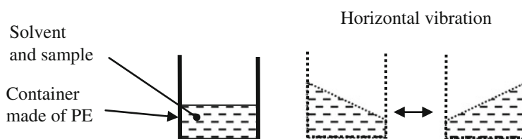
Fig. 2 Schematic of leaching test based on public announcement no. 19 of the Environment Agency in Japan
