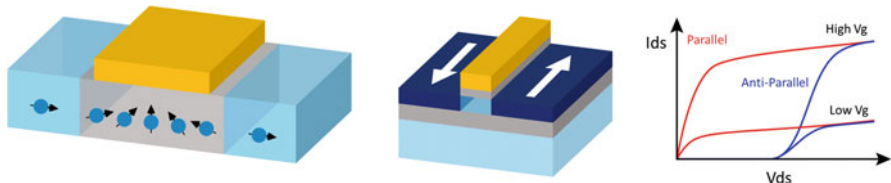
Fig. 4 Spin-based processing device with memory function (left: Spin FET; middle: Spin MOSFET; right: expected I–V characteristics)
