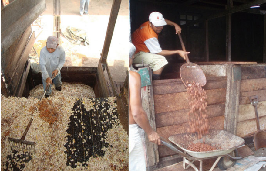
Fig. 3.1 Cocoa bean box fermentation is a commonly used method for fermentation of the cocoa pulp-bean mass. A cascade of three boxes of about 1 m 3 each is an optimal setup for this fermentation process. In a box fermentation process, fermentation of the cocoa pulp-bean mass starts in the upper box; every 24 h, the fermenting cocoa pulp-bean mass is transferred to a lower box. At the end of the fermentation process, the fermented cocoa beans are collected
