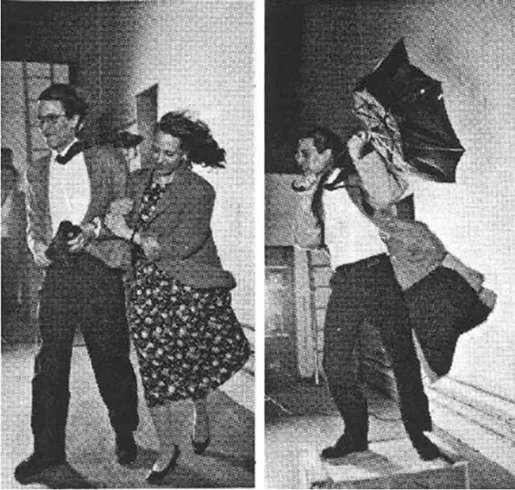
Fig. 6.8 Wind tunnel exposure of people at 70 km/h winds
