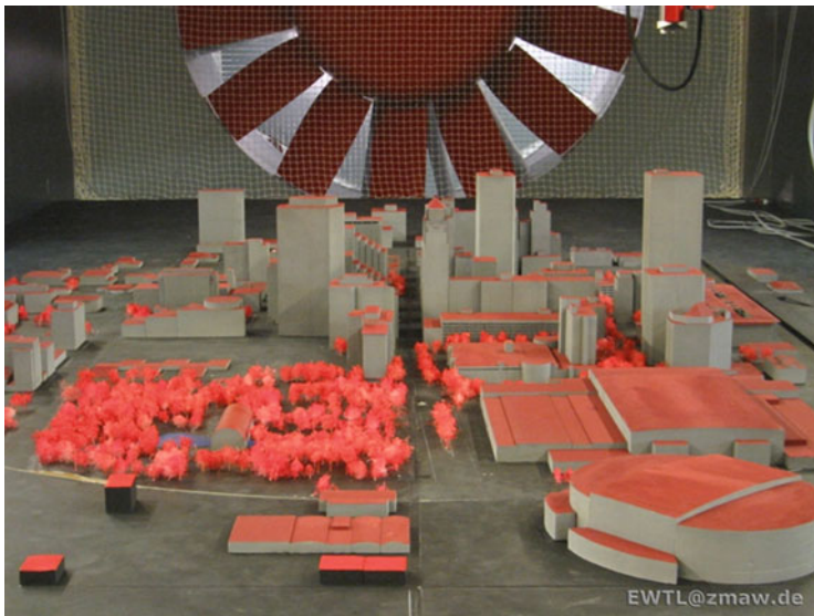
Fig. 8.3 Wind tunnel model of the Central Business District of Oklahoma City
