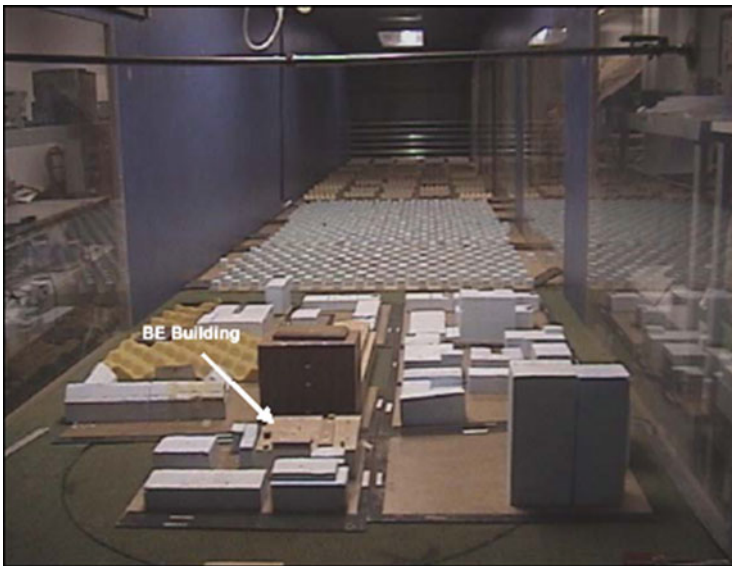
Fig. 6.11 Typical wind tunnel setup for a pedestrian wind assessment study in the atmospheric boundary layer wind tunnel at Concordia University, Montreal
