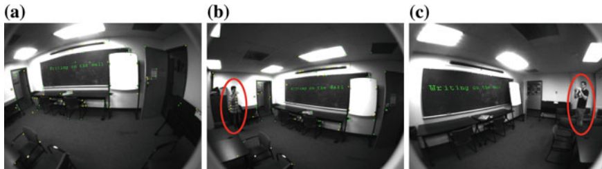
Fig. 5 Client 1 created a map with virtual text. Clients 2 and 3 simultaneously downloaded the map, including the virtual text. Clients 2 and 3 are circled in each other’s images for perspective. a Client 1. b Client 2. c Client 3
