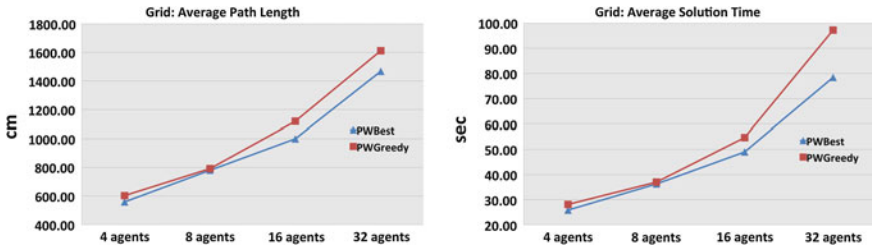
Fig. 10 The average path length and average time to finish for simulations using the polynomial weight with greedy (PWGreedy) and with k-best selection (PWBest)
