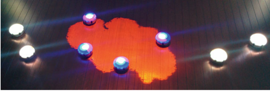
Fig. 1 A visual representation of the collaboration experiment firefighting scenario using the Droplet swarm robotic platform
