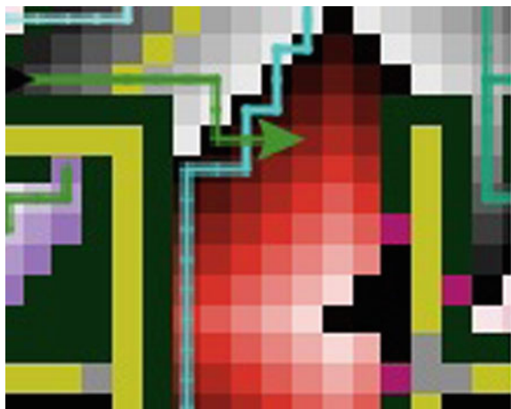
Fig. 4 Marsu using splash algorithm for reaching its goal, in this figure yellow patches are already discovered walls, gray ones undiscovered walls, green ones discovered space evaded by algorithm and the gradient colored ones are the ones showing how the algorithm works by coloring the value of the patch splash value, these are colored for illustration purposes only
