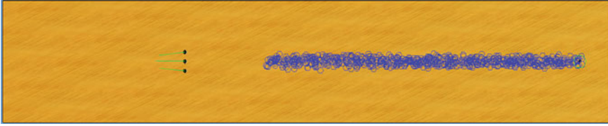
Fig. 2 Simulation setup, with the source on the right and robots starting on the left . The plume is shown in blue , and consists of filaments with growth rate \gamma = 4 \times 10^{-7} \text{ m}^2 \text{ s}^{-1} . The wind flows right-to-left . For ease of visualization, the filaments are drawn enlarged
