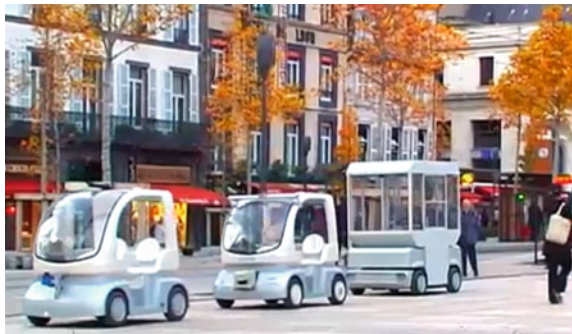
Fig. 1 Autonomous navigation in formation of a group of UGVs in an urban environment (Clermont-Ferrand, France)
