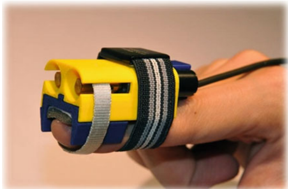
Fig. 6.8 Gravity grabber in use
