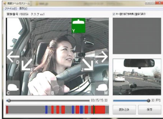
Fig. 3.3 Labeling of gaze direction. We labeled driver gaze direction with tags, using the lane change driving data mentioned above. A gaze direction labeling tool was developed which can classify gaze direction into one of 10 categories based on video images of drivers faces. We used the collected driving data and gaze label data to successfully model the relationship between driver gaze behavior and driving behavior
