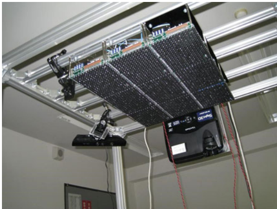
Fig. 5.15 Airborne ultrasound tactile display with 3 by 3 units [7]. The size of a unit is 19 \times 15 \text{ cm}^2
