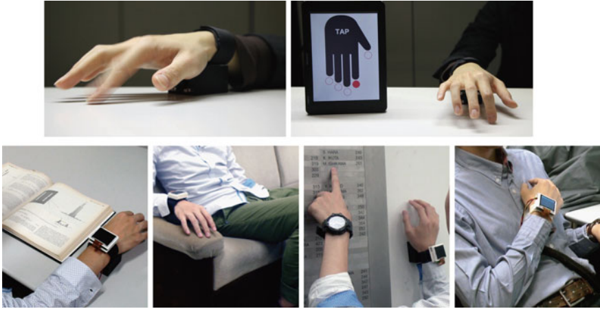
Fig. 5.36 Anywhere surface touch: utilizing any surface as an input area with a wearable device [37]
