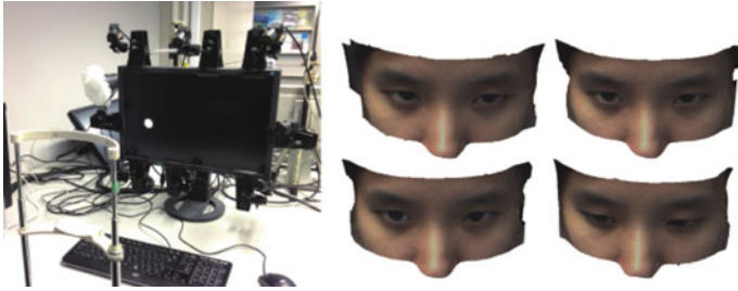
Fig. 8.6 Data collection. Left System configuration for data collection. Right Examples of reconstructed 3D eye region models (Reproduced with permission of © 2014 IEEE [45])
