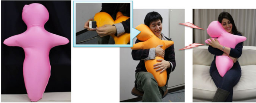
Fig. 2.4 Hugvie™. A user inserts his/her smartphone in a pocket at Hugvie’s head and talks by hugging it
